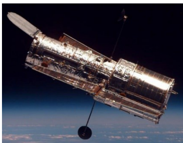
The Hubble Space Telescope has a 2.4m diameter collecting mirror.
